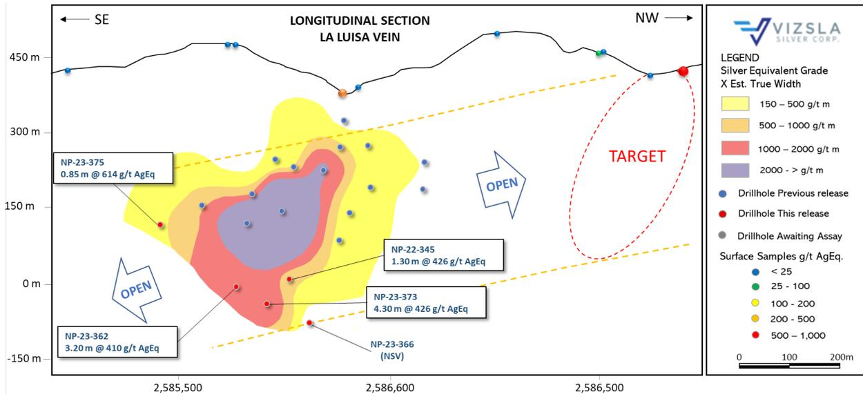
**Figure 2:** Longitudinal section of the La Luisa Vein.
