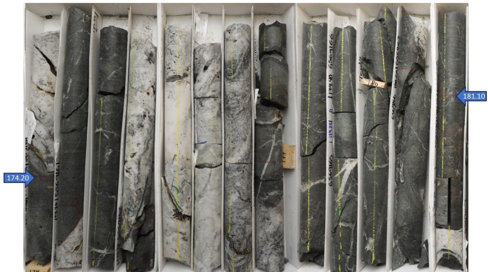
Figure 5: Photo of NP-23-411 showing El Molino vein from 174.20 to 181.10 metres down the hole. Disseminated and semi-massive sulfides occur down to 181.10 metres.
