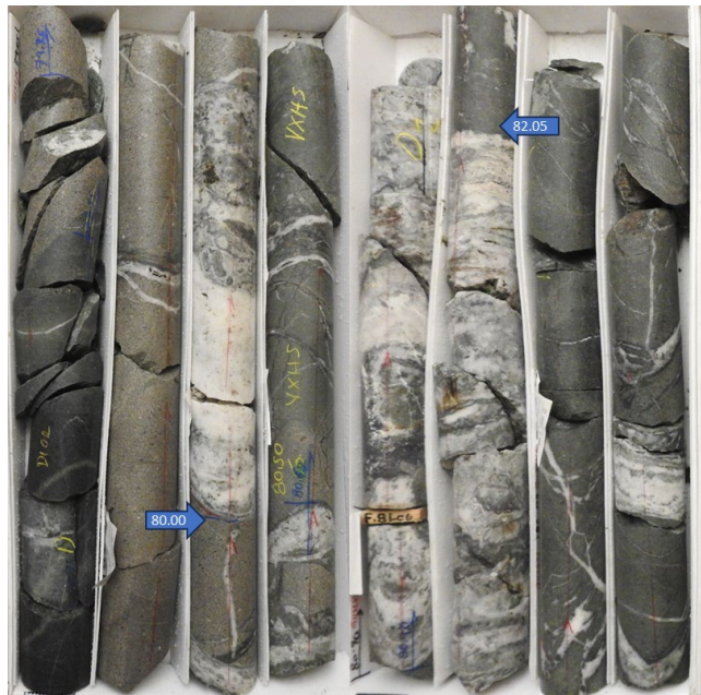
Figure 4: Photo of NP-23-359 showing El Molino vein from 80.00 to 82.05 metres down the hole.
