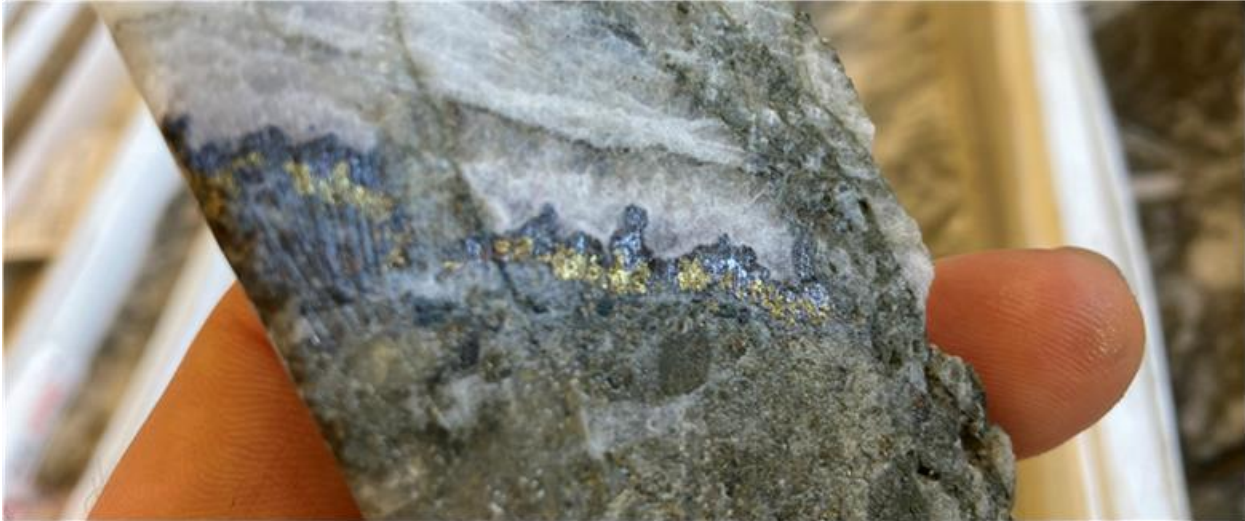
Figure 12-6 A) Core from Drillhole CS-22-169 (Sulfide Minerals Visible with Metallic Lustre) and B) Core from Drillhole NP-22-300 (Silver Mineralisation Visible in Grey)
